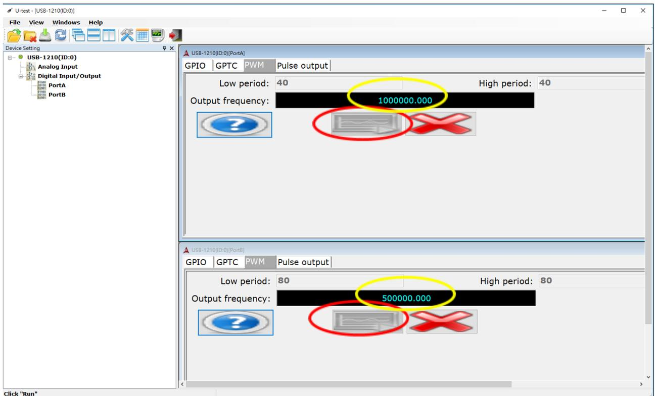
$$F_{PWM} = \frac{F_{Timebase}}{Pulse\_initial\_cnt + Pulse\_length\_cnt}$$
