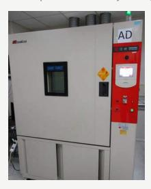
/Temperature testing/ -60°C to +150°C
